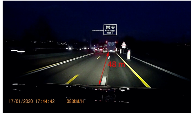
Figure 1. An example where geometric calibration is required is the distance analysis in automotive imaging.
