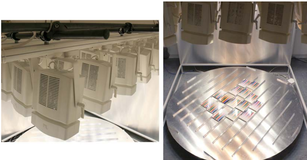
Figure 6: Light fading lamp unit and rotating sample area
