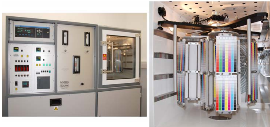
Figure 9: Ozone Test Chamber, Satra-Hampden Model 903 and internal test chamber with rotating test piece carrier
