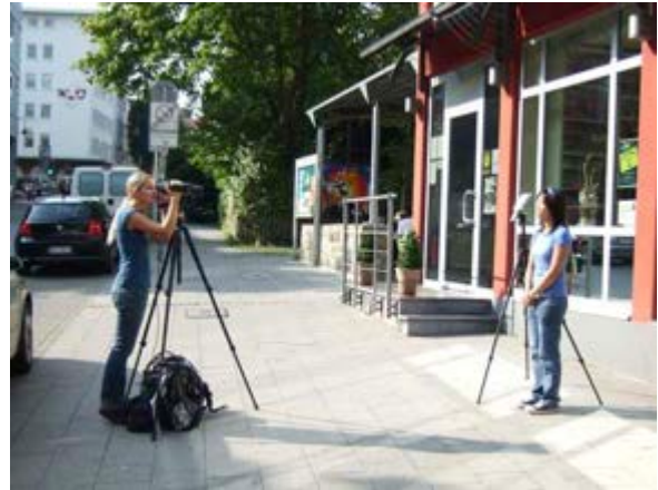
Figure 14: Telespectroradiometer at camera position measuring scene elements.
