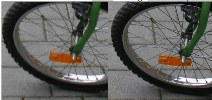
20. Figure: In the image on the right the object is in focus. On the left side the focal plane is far behind the object.
