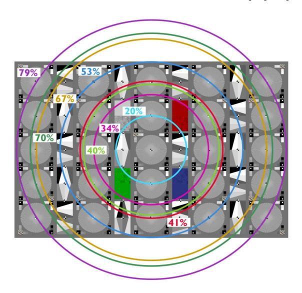
The maximum resolution of the TE268 A depends on chart size and diameter of the center mark:
