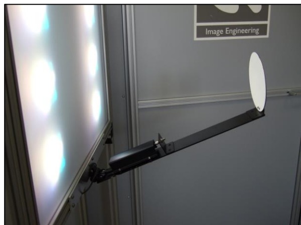
The calibration device is in the "measure position."
