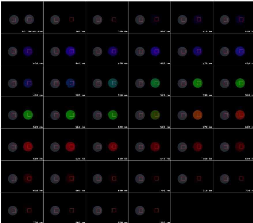
Figure 4.5.1: A tiled image is created from all images of a series for camSPECS multi-shot. Displaced filter frames can easily be identified.
