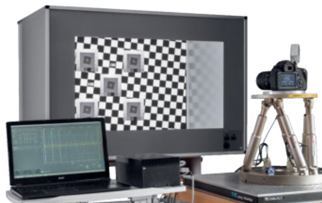
OIS test with the STEVE 6DL and the iQ-AF Box
