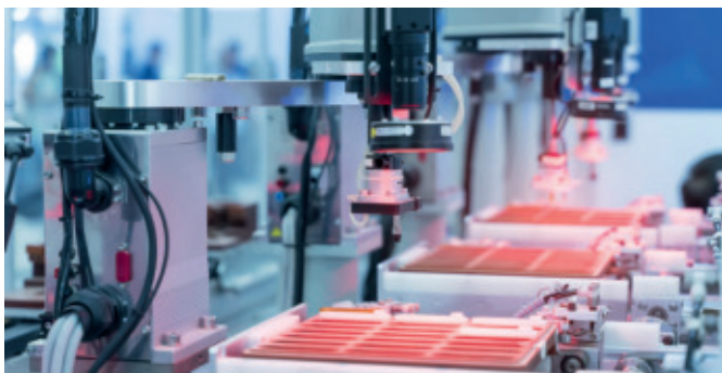
Calibrate multiple camera modules at the same time on a production line.
